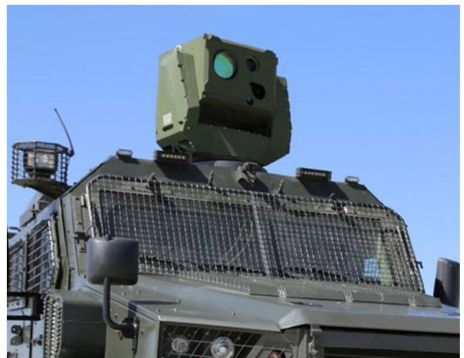
Turkish Laser Defense System, developed by Aselsan, is mounted on a military vehicle. (Image Credit: Aselsan)
