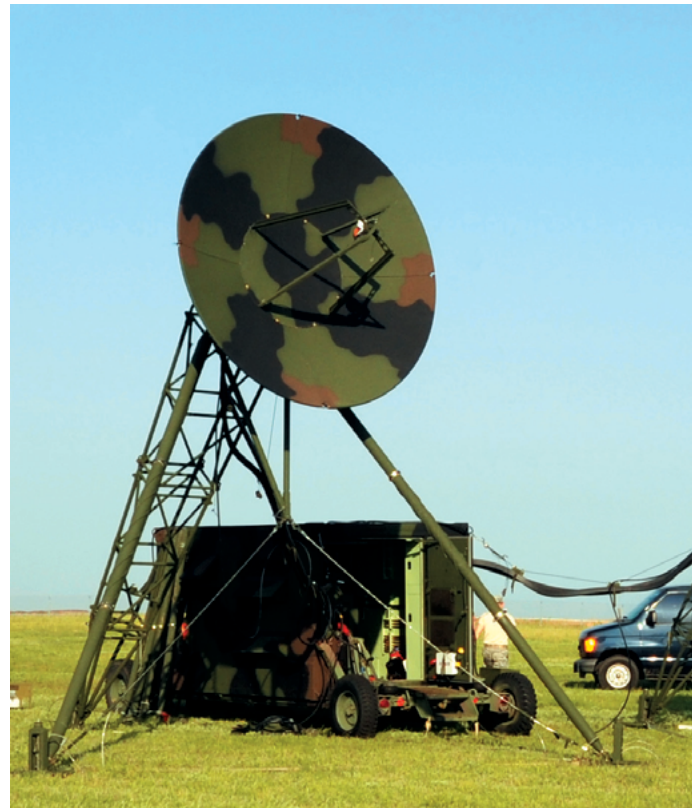
A Tropospheric Scatter Microwave Radio Terminal (TRC-170) from the 31st Combat Communication Squadron, Tinker Air Force Base, Okla., is positioned in a field during an exercise on May 1, 2012.
