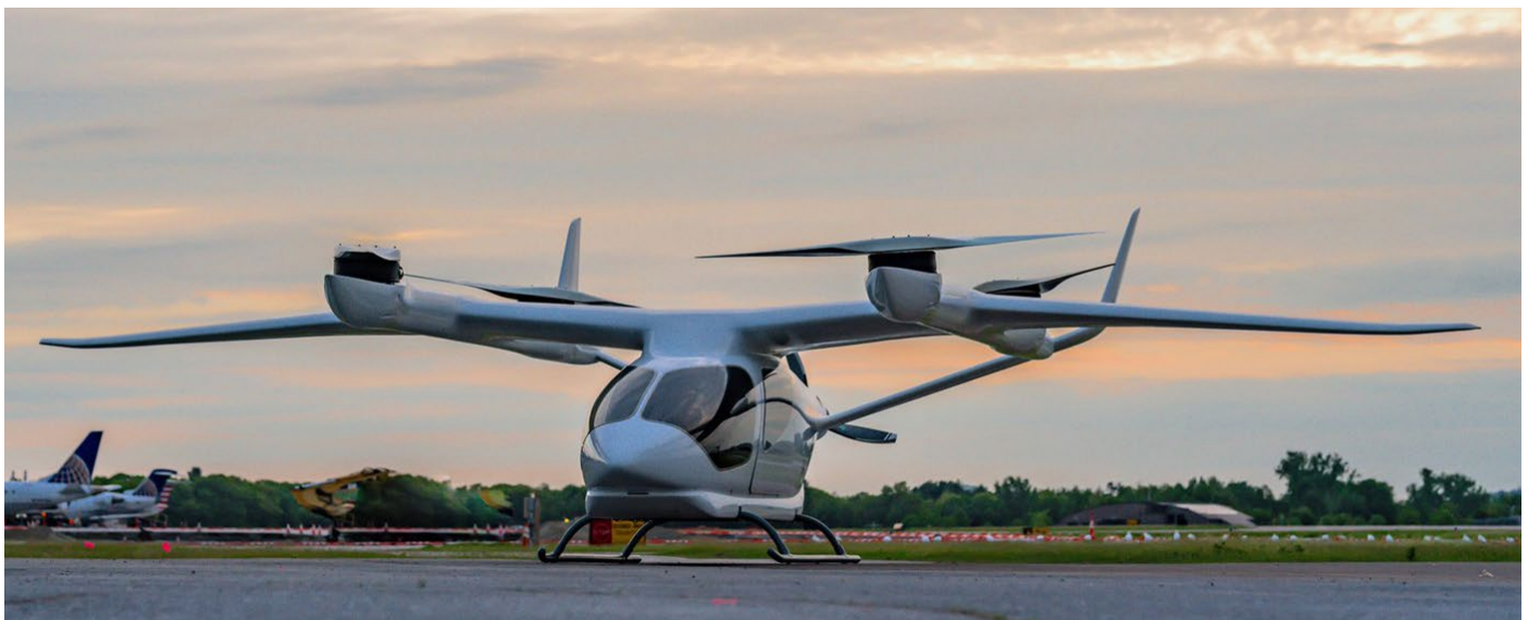
Beta Technologies ALIA-250 electric conventional takeoff and landing aircraft. (Image Credit: Eric Adams/Electric VTOL News)
