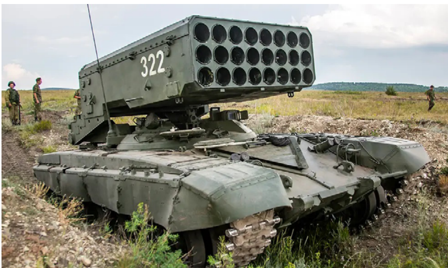
A BM-1 launcher from a TOS-1A system of the Russian 1st Mobile NBC Protection Brigade at the Shikhany proving ground. (Image Credit: Yevgeny Kel/Russian Ministry of Defense)
